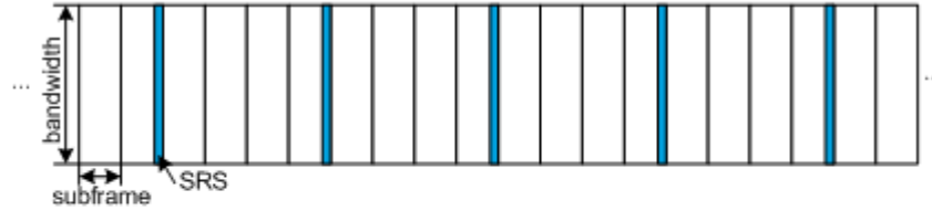
SRS transmission with frequency hopping ( B_{\text{SRS}} \neq 0 )
